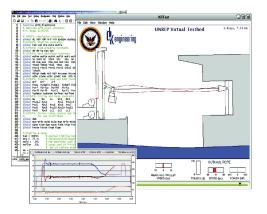
The UVTB provides simulated strip-chart output of system parameter values (speeds, tensions, etc.), twodimensional animations of simulated cargo operation, and tabular numeric output of all pertinent system variables versus time. D&K Engineering used this tool to perform dozens of simulated at-sea tests, drastically reducing development time, prompting specific improvements in hardware and software, and increasing the client's
